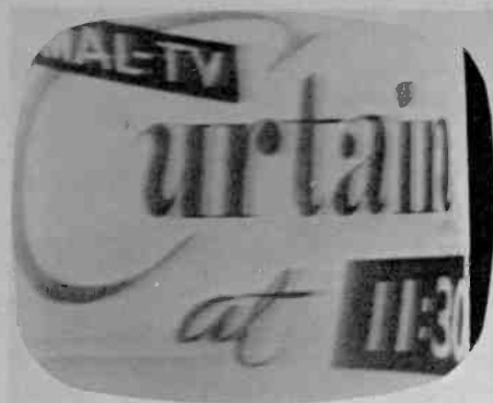
FIG. 14. Loss of width due to an open capacitor at output of damper filter.
