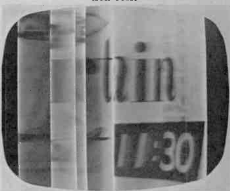
FIG. 13. Distortion due to an open capacitor at input of damper filter.
