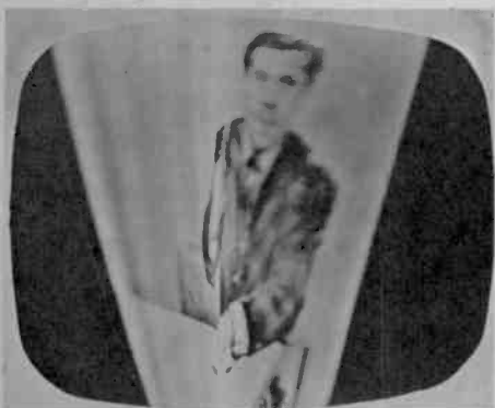
FIG. 11. Keystoning effect of shorted horizontal yoke.
