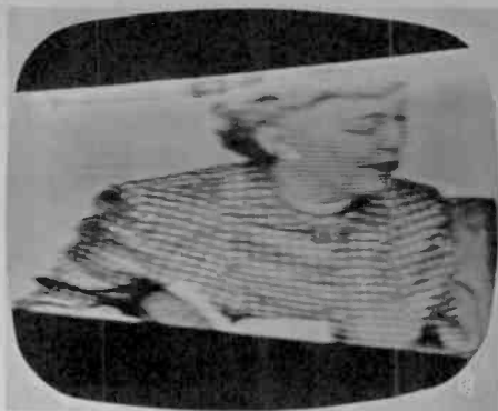
FIG. 12. Trapezoidal sweep resulting from a short across one section of vertical deflection coil.
